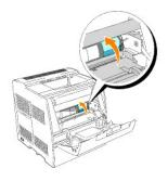
3. Hold the toner cartridge and pull out the cartridge.
