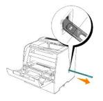
3. Push the two tabs on the cleaning pad inward to remove the pad.
