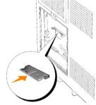
5. Reattach the control board cover to the printer.
