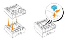
7. Place the printer on top of the tray module(s).
