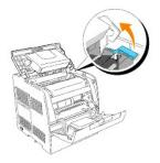
3. Grab the drum cartridge by the handle, and pull it up and out.
