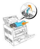
3. Pull down the lever on the right to lock the drum cartridge in place.
