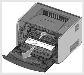
**5** Open the rear exit and remove any jams.
