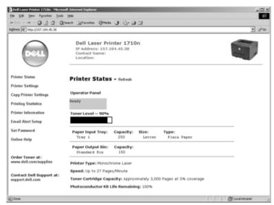
You can set up the Dell Printer Configuration Web Tool to send you an email when the printer needs supplies or intervention.
