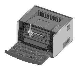
**3** Pull the toner cartridge up and out using the handle.
