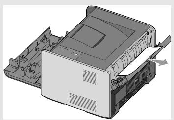
6 After you have cleared the jams, reinstall the toner cartridge assembly, make sure all printer covers and trays are closed, and then press **Continue** (b) to resume printing.
