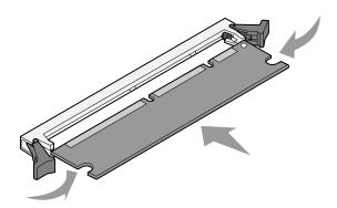
**7** Push the memory card firmly into the connector until the latches on either end of the connector *snap* into place.
