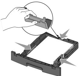
If you are loading legal or folio size paper, press down on the latch at the back of the tray and expand the tray until the extender locks into place.
