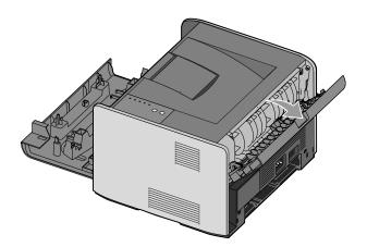
3 Open the side cover by pressing the two detents on the front right side of the machine and swinging the cover back.
