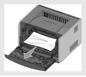
**4** Lift the flap at the front of the printer and remove any jams beneath the flap.
