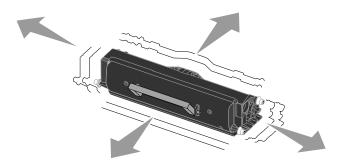
**6** Install the new toner cartridge by aligning the white rollers on the toner cartridge with the white arrows on the tracks of the imaging drum and pushing the toner cartridge in as far as it will go. The cartridge *clicks* into place when correctly installed.
