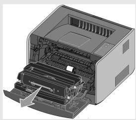
**NOTE:** Do not leave the toner cartridge assembly exposed to direct light for an extended period of time. Extended light exposure can cause print quality problems.
