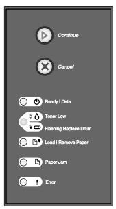
When the **Toner low** light sequence appears or when you experience faded print, remove the toner cartridge. Firmly shake it side-to-side and front-to-back several times to redistribute the toner, and then reinsert it and continue printing. Repeat this procedure multiple times until the print remains faded. When the print remains faded, replace the toner cartridge.
