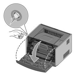
CAUTION: When replacing a toner cartridge, do not leave the new cartridge exposed to direct light for an extended period of time. Extended light exposure can cause print quality problems.
