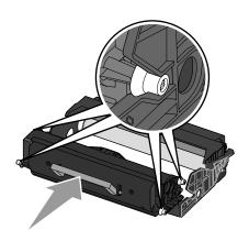
7 Install the toner cartridge assembly into the printer by aligning the blue arrows on the guides of the toner cartridge assembly with the blue arrows on the tracks in the printer and pushing the toner cartridge assembly in as far as it will go.
