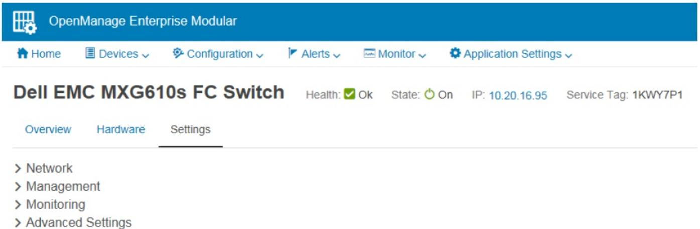
4. Click and expand the **Network** option. Select the required check boxes, and complete the IPv4 or IPv6 settings, DNS server settings, and optionally the management VLAN ID. Click **Apply**.
