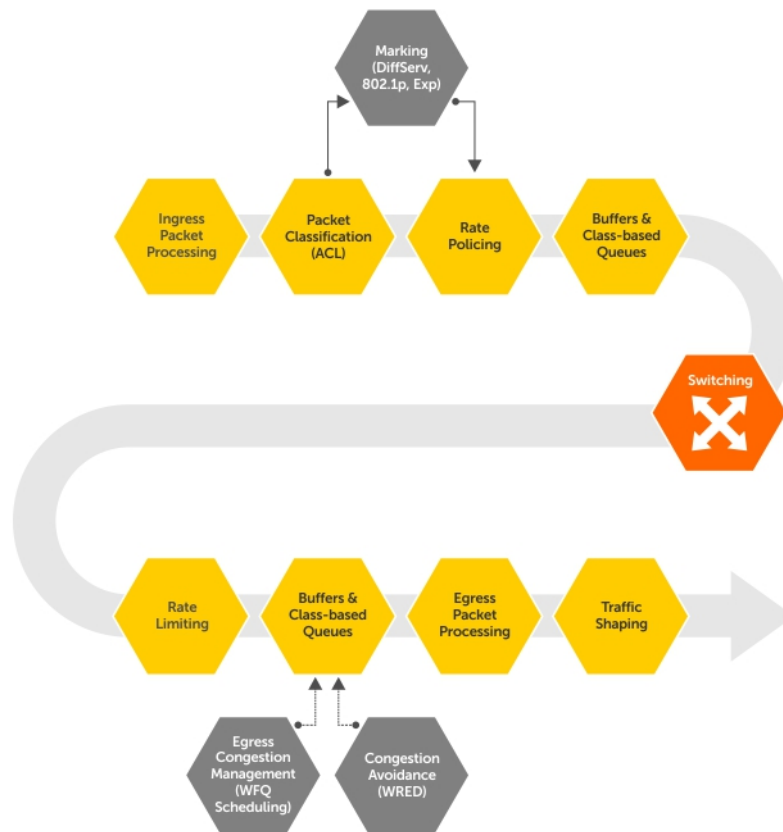
Figure 109. Dell EMC Networking QoS Architecture
