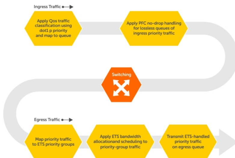
Figure 32. DCB PFC and ETS Traffic Handling
