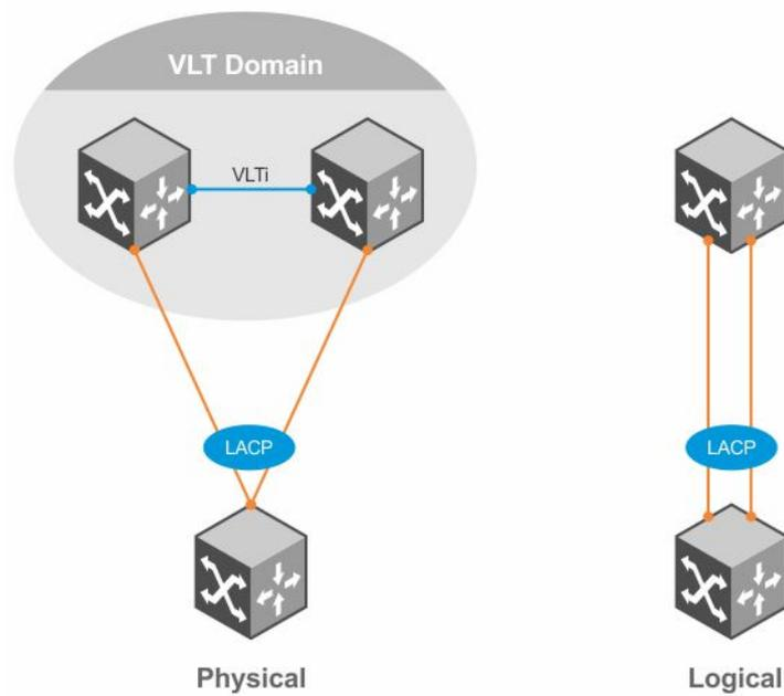
**Figure 127. VLT providing multipath**
