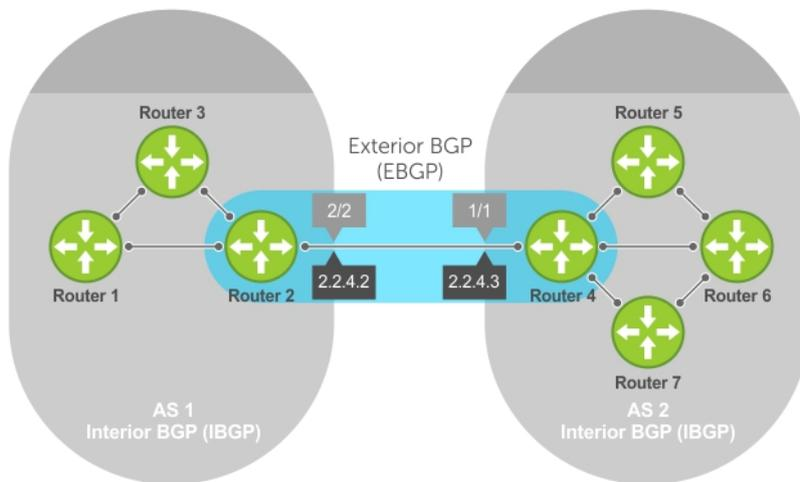
**Figure 17. BGP Topology with autonomous systems (AS)**
