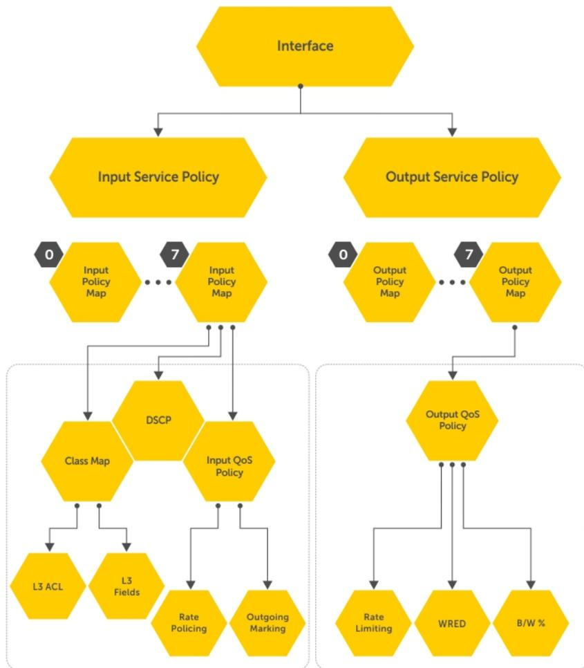
Figure 103. Constructing Policy-Based QoS Configurations
