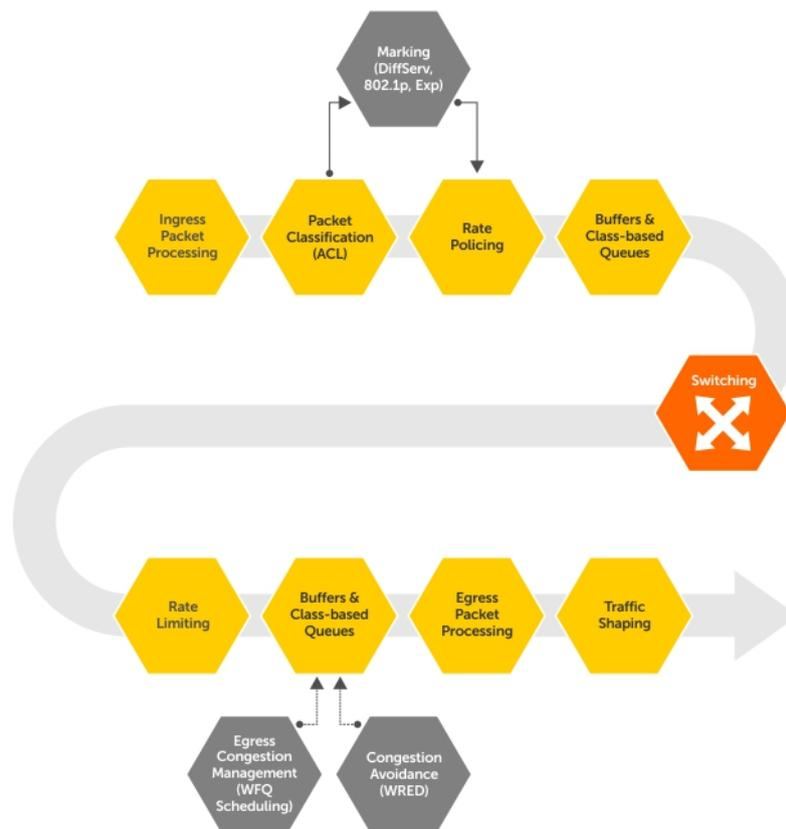
**Figure 102. Dell EMC Networking QoS Architecture**
