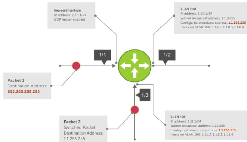
Figure 46. UDP Helper with Configured Broadcast Addresses
