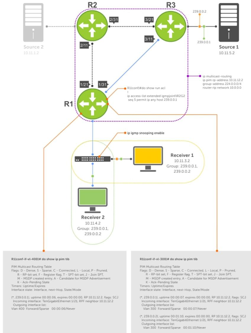
**Figure 39. Preventing a Host from Joining a Group**
