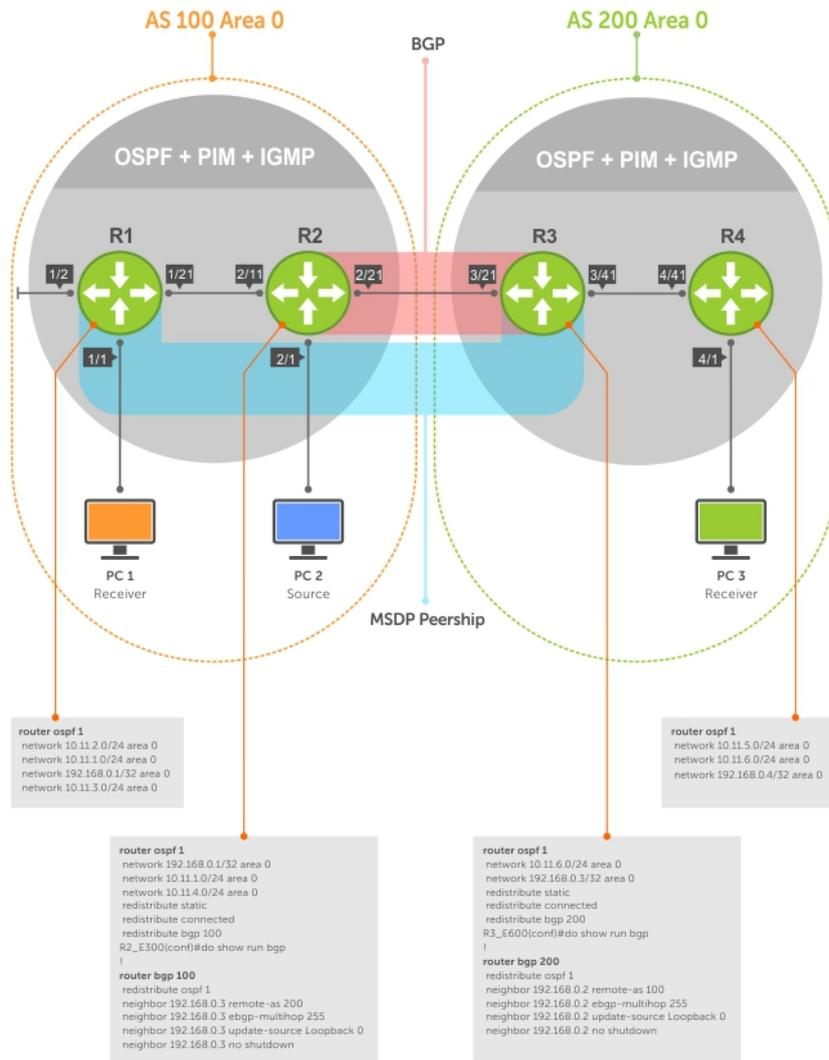
Figure 77. Configuring OSPF and BGP for MSDP
