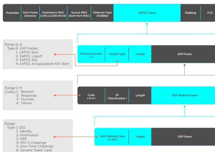
Figure 4. EAP Frames Encapsulated in Ethernet and RADIUS
