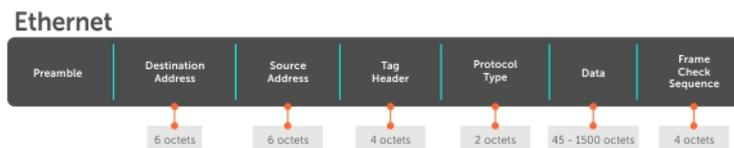
Figure 125. Tagged Frame Format
