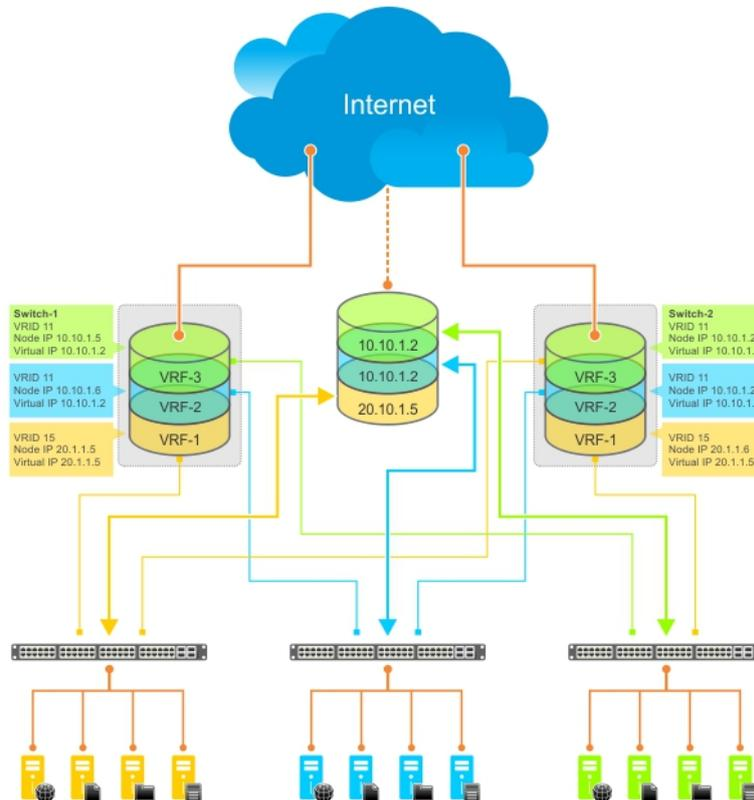
Figure 148. VRRP in a VRF: Non-VLAN Example
