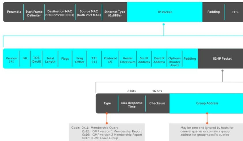
Figure 34. IGMP Messages in IP Packets
