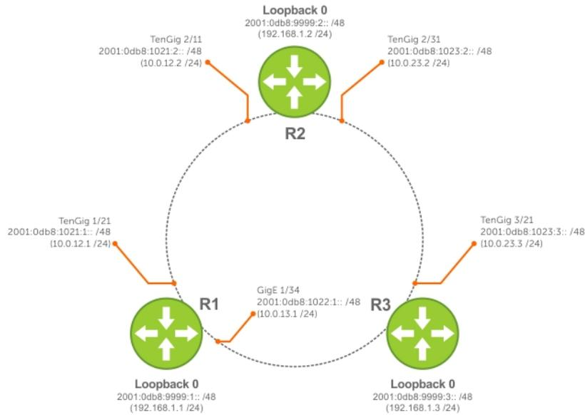
**Figure 52. IPv6 IS-IS Sample Topography**
