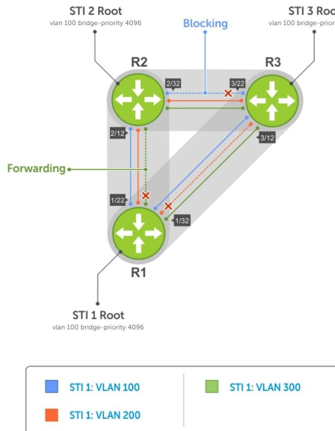
**Figure 100. Load Balancing with PVST+**
