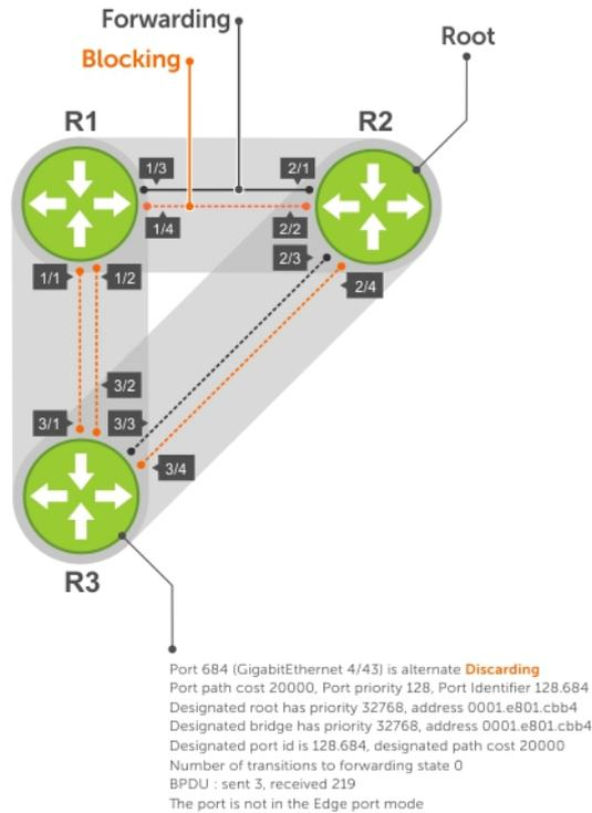
**Figure 106. Rapid Spanning Tree Enabled Globally**
