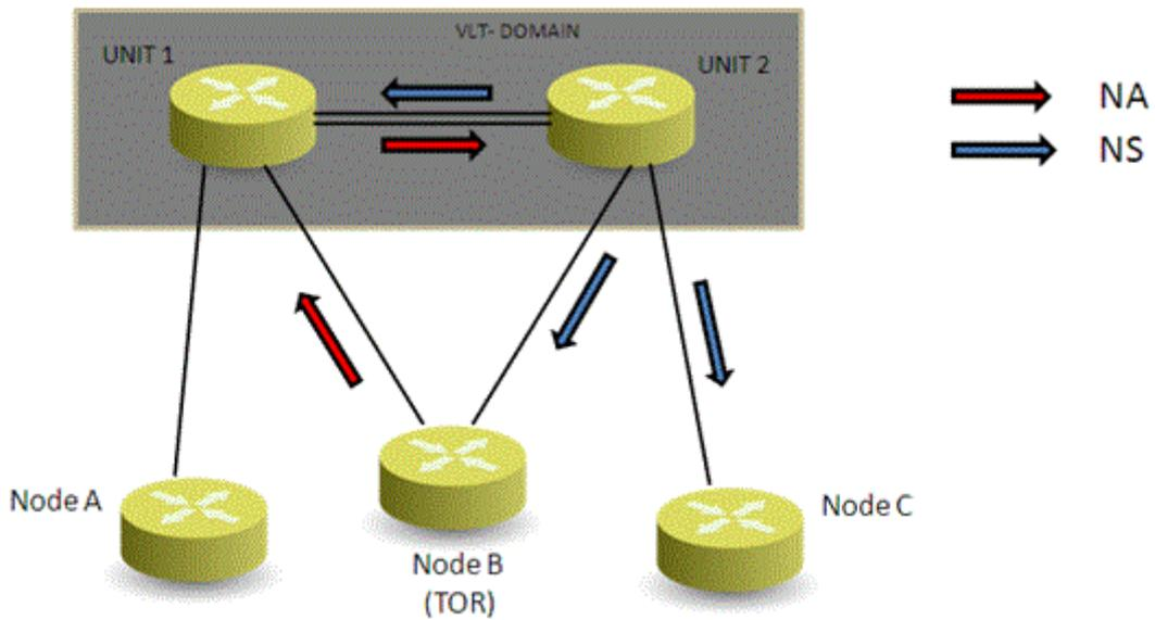
Figure 137. Sample Configuration of IPv6 Peer Routing in a VLT Domain
