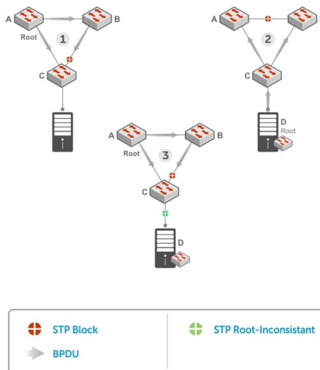
Figure 119. STP Root Guard Prevents Bridging Loops
