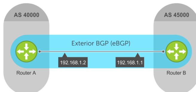
Figure 23. BGP topology with two AS
