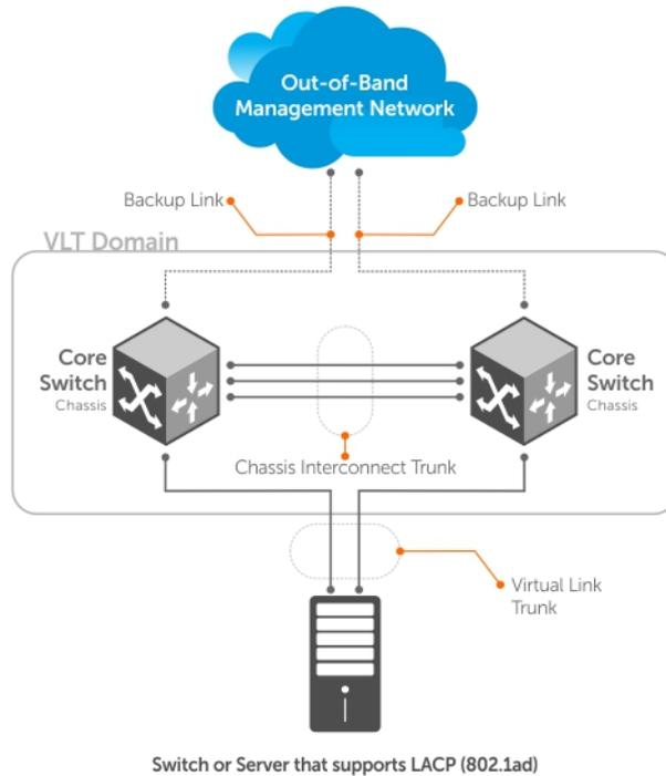
**Figure 128. Example of VLT Deployment**
