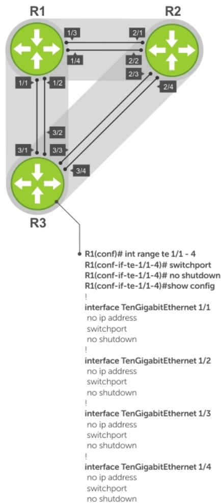
**Figure 116. Example of Configuring Interfaces for Layer 2 Mode**
