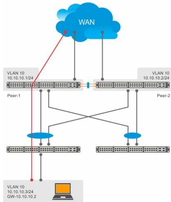
**Figure 134. Packets with peer routing enabled**
