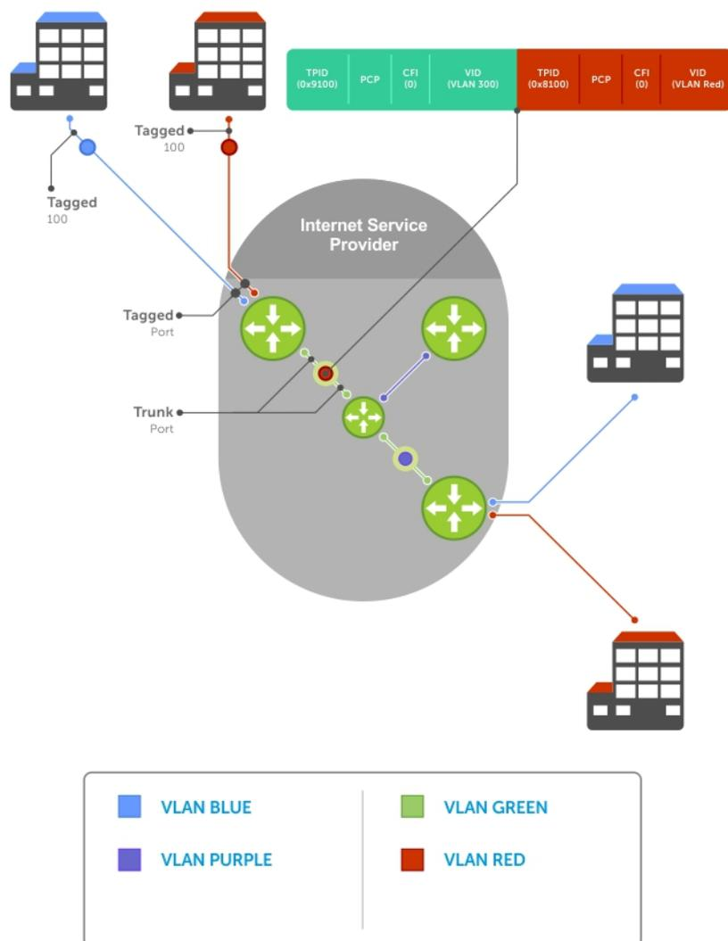
**Figure 107. VLAN Stacking in a Service Provider Network**
