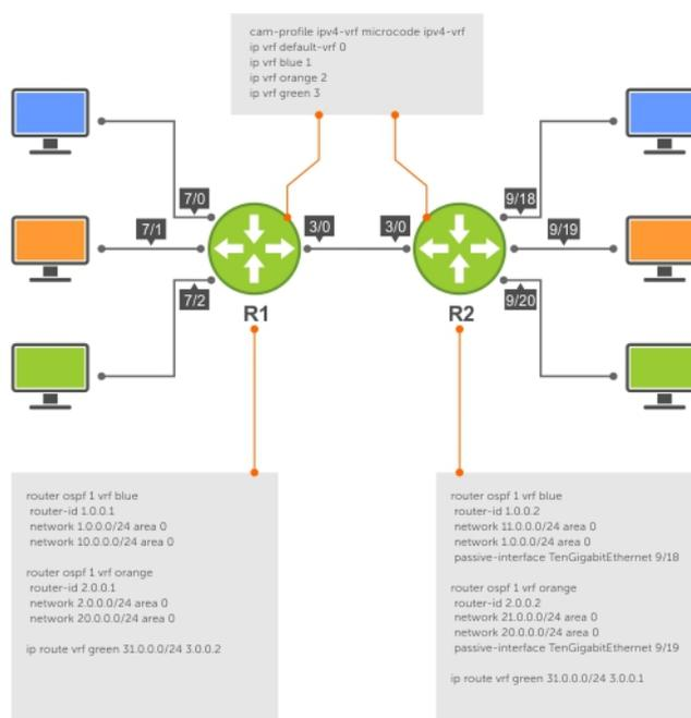
Figure 143. Setup OSPF and Static Routes
