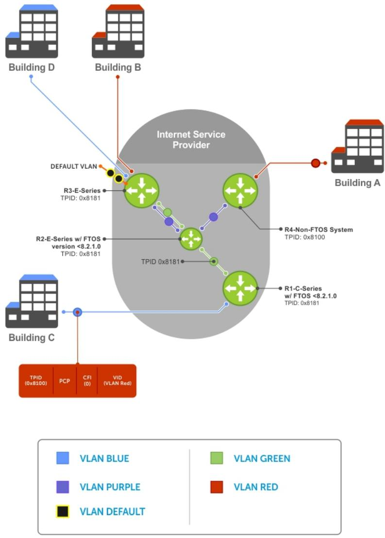
Figure 109. Single and Double-Tag First-byte TPID Match
