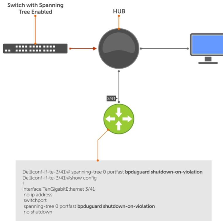
**Figure 118. Enabling BPDU Guard**
