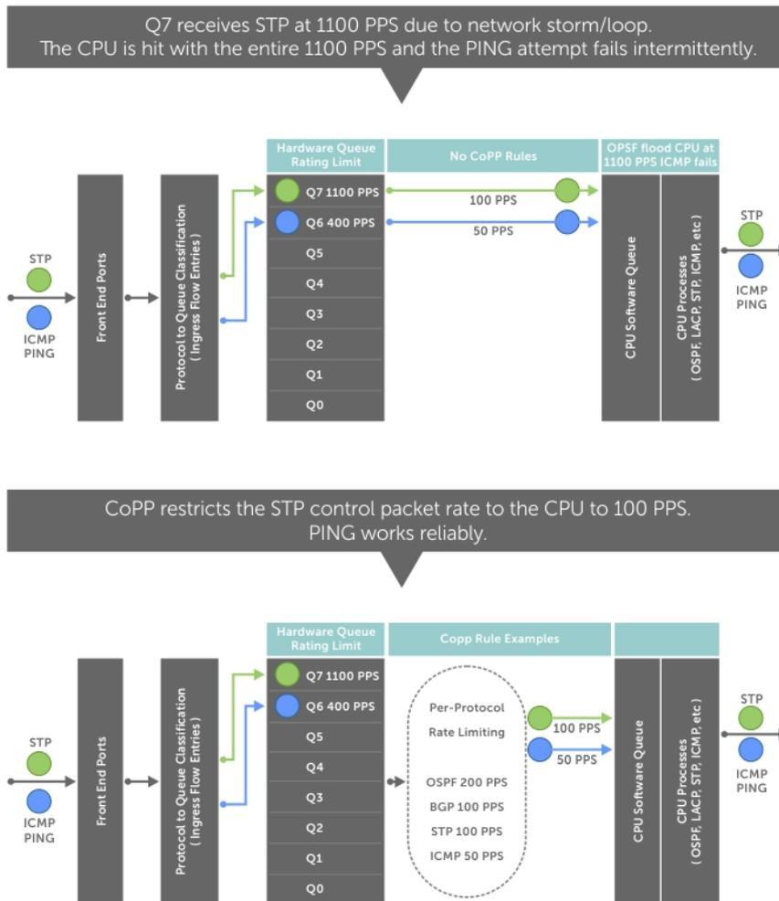
**Figure 28. CoPP Implemented Versus CoPP Not Implemented**
