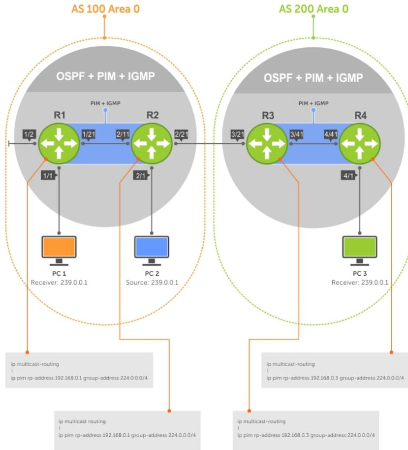
Figure 78. Configuring PIM in Multiple Routing Domains
