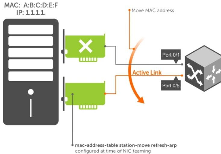
**Figure 63. Configuring the mac-address-table station-move refresh-arp Command**
