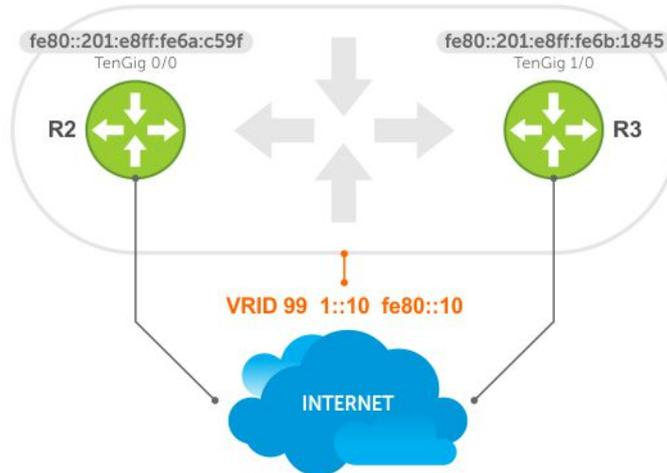
**Figure 147. VRRP for an IPv6 Configuration**
