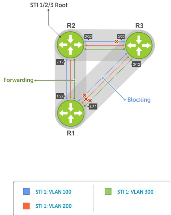
**Figure 99. Per-VLAN Spanning Tree**
