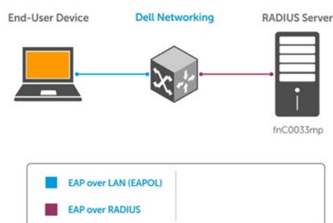
Figure 3. EAP Frames Encapsulated in Ethernet and RADIUS
