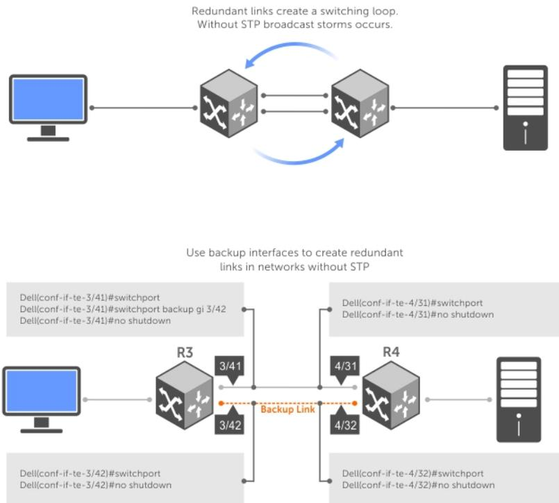
**Figure 64. Configuring Redundant Layer 2 Pairs without Spanning Tree**
