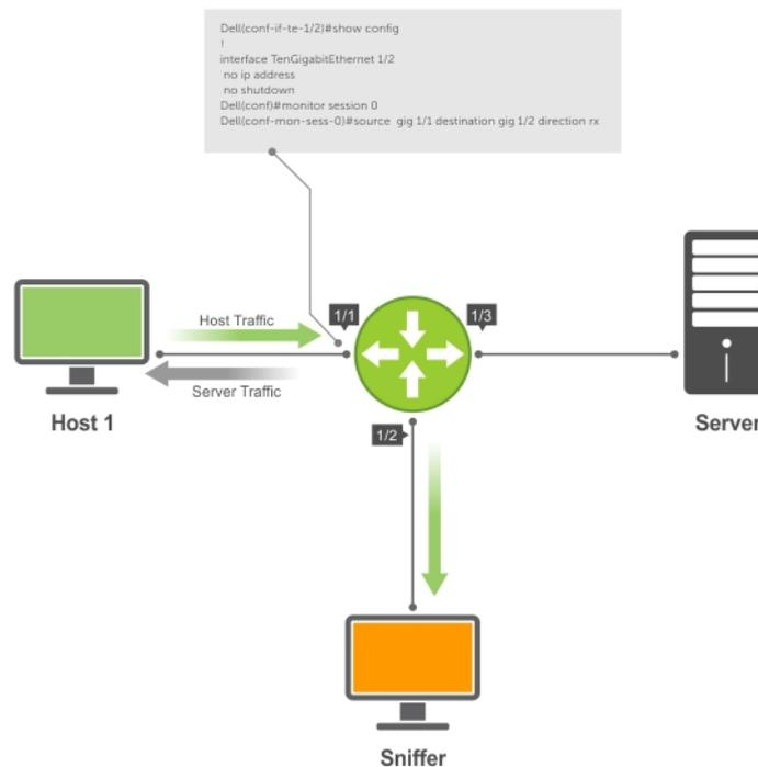
Figure 94. Port Monitoring Example
