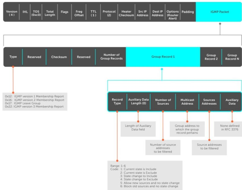
Figure 36. IGMP Version 3-Capable Multicast Routers Address Structure
