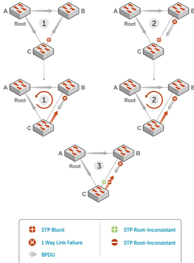
Figure 120. STP Loop Guard Prevents Forwarding Loops
