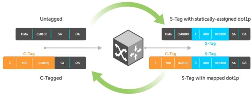
**Figure 111. Statically and Dynamically Assigned dot1p for VLAN Stacking**
