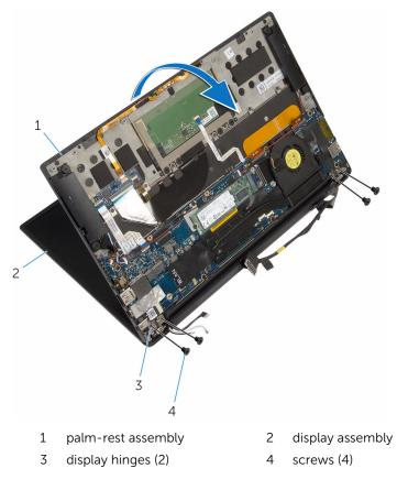
**15** Slide and remove the palm-rest assembly from the display hinges.
