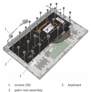
4 Lift the keyboard off the palm-rest assembly.
