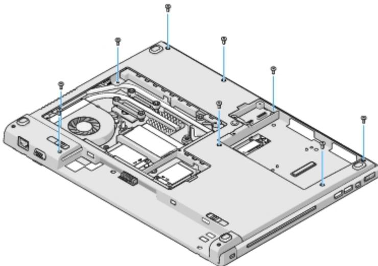
9. Turn the computer over and remove the eight M2.5 x 5-mm screws that secure the top of the palm rest. Use the "P" symbols located on the palm rest to assist in finding the screw locations.
