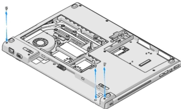
7. With the computer facing top side up, remove in sequential order the three numbered M2.5 x 5-mm screws from the base of the display assembly.
