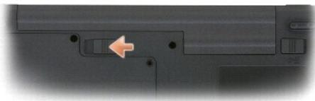
4. Slide the right battery-bay latch release and slide the battery out of the battery bay.
