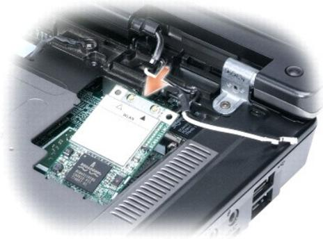
2. Press the other end of the Mini-Card into the securing tabs until the card clicks into place.
