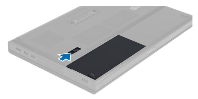
3. Flip and remove the battery from the computer.
