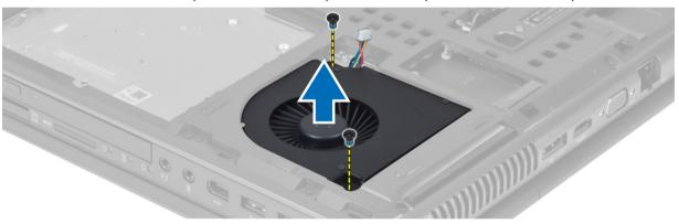
4. Disconnect the processor-fan cable.
