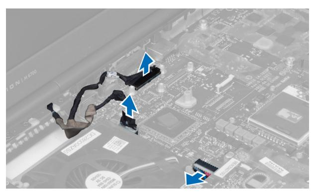
6. Disconnect the switch board cable from the system board.
