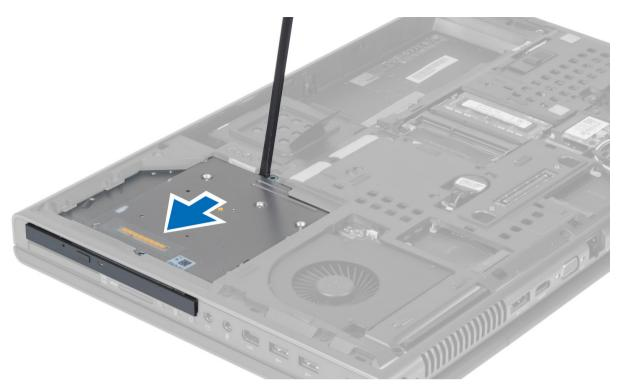
5. Remove the screws that secure the drive-latch bracket to the optical drive and remove the bracket.
