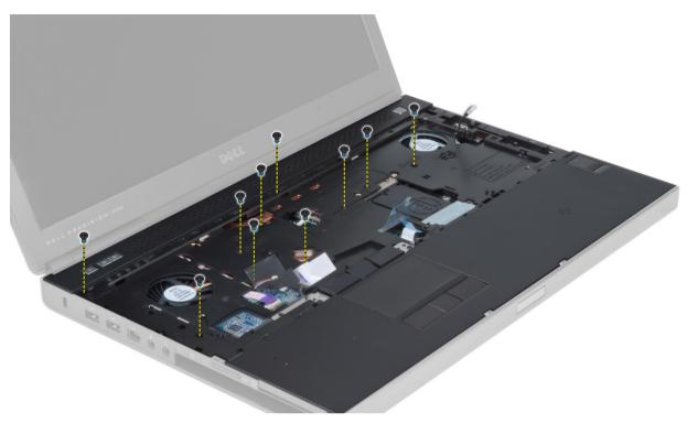
13. Lift the left edge of the palmrest. Release the tabs on the right edge of the palmrest and remove the palmrest from the computer.
