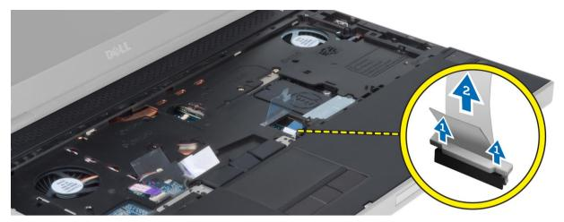
$\textbf{10.} \quad \text{Disconnect the power button cable from the system board}.$
