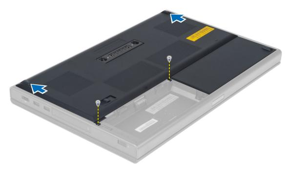
4. Flip and remove the base cover from the computer.
