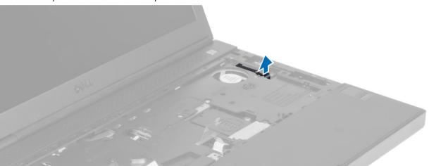
11. Disconnect the bluetooth module cable from the system board.
