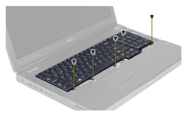
4. Starting from the bottom of the keyboard, separate the keyboard from the computer and flip the keyboard over.
