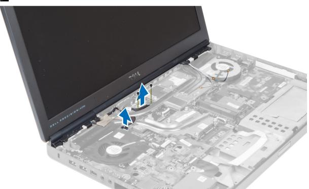
Remove the screws that secure the display assembly to the computer. Remove the display assembly from the computer.
