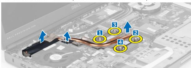
4. Remove the heat sink from the computer.
