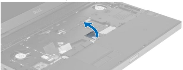
9. Disconnect the touchpad cable from the system board.
