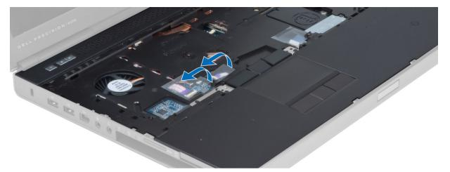
$\textbf{7.} \quad \text{Disconnect the media board cable and the speaker cable from the system board.}$
