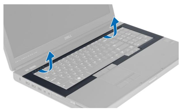
**4.** Pry up the bottom edge of the keyboard trim from the top-inner edge.
