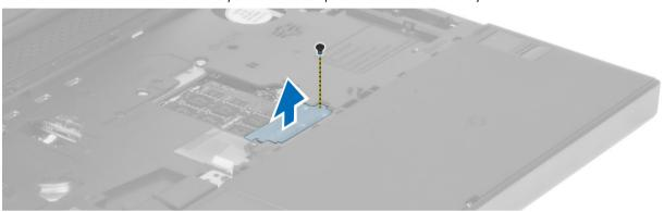
4. Pry the retention clips away from the memory module until it pops up. Lift up the memory module and remove it from the computer.
