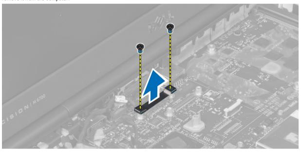
$\textbf{5.} \quad \text{Disconnect the LVDS , camera and power connector cables from the system board.}$
