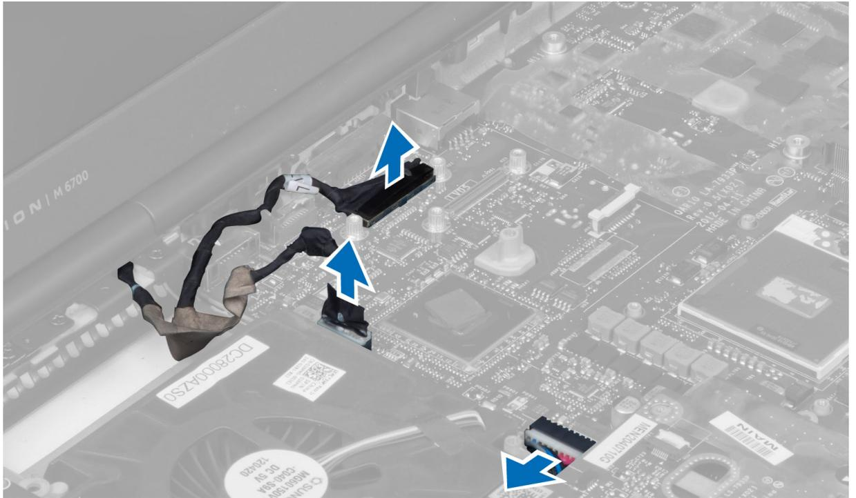
6. Disconnect the switch board cable from the system board.
