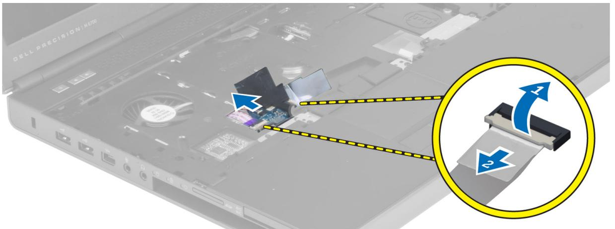
8. Peel the adhesive tape that secures the touchpad cable to the palmrest.
