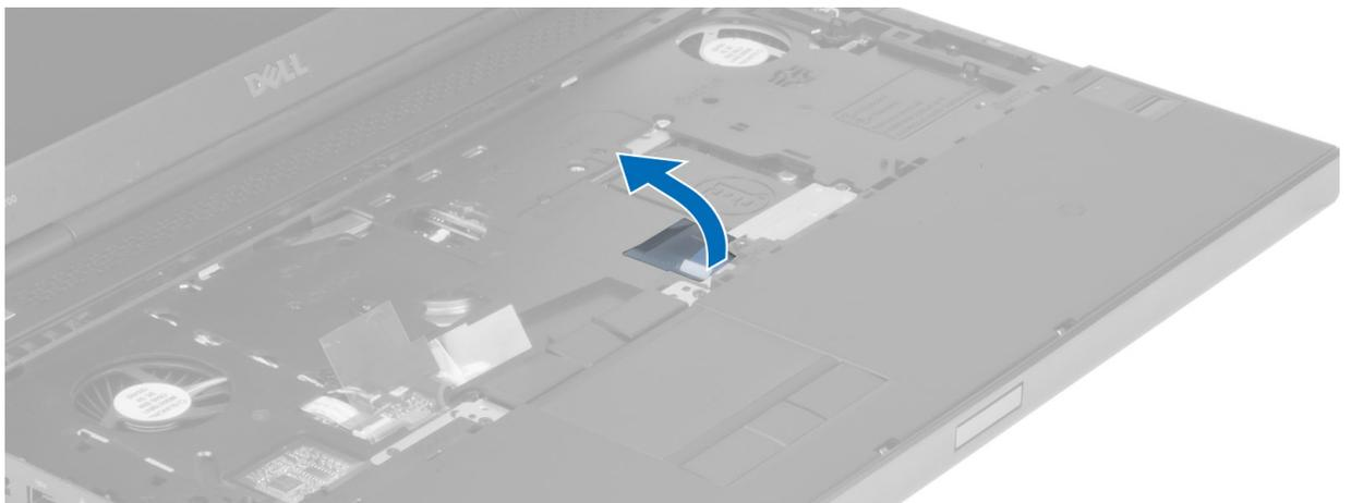
9. Disconnect the touchpad cable from the system board.
