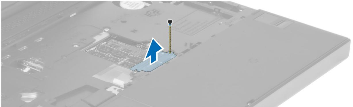
4. Pry the retention clips away from the memory module until it pops up. Lift up the memory module and remove it from the computer.
