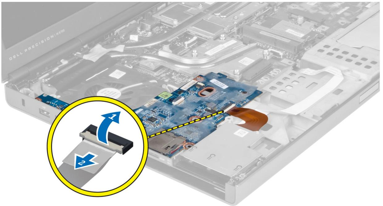
4. Remove the screw that secures the I/O board to the computer. Lift the right edge of the I/O board upwards to disengage the connector and remove it from computer.
