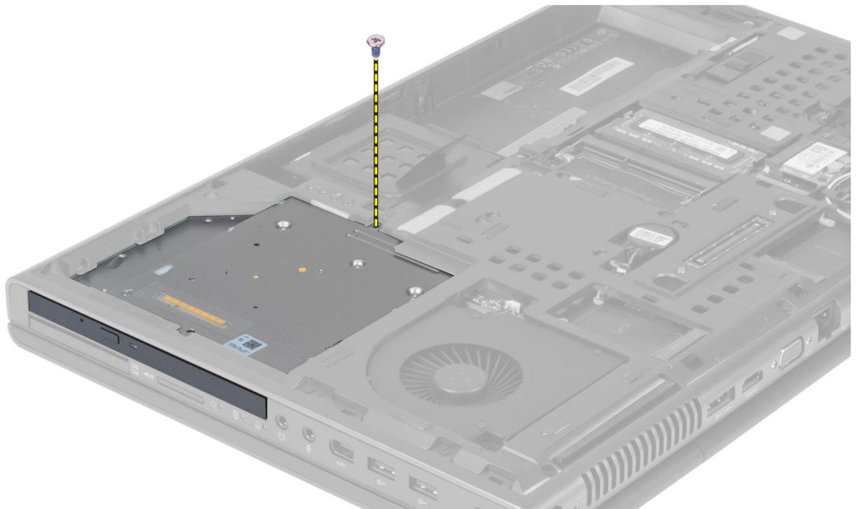
4. Pry and slide out the optical drive to remove it from the computer.
