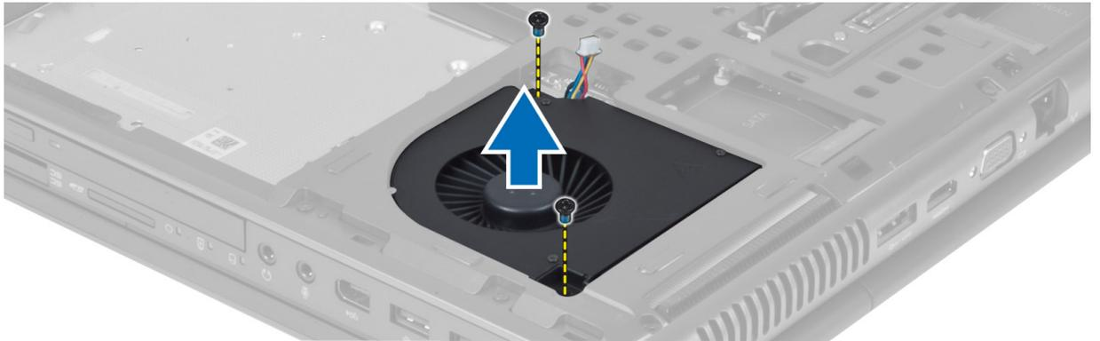
4. Disconnect the processor-fan cable.
