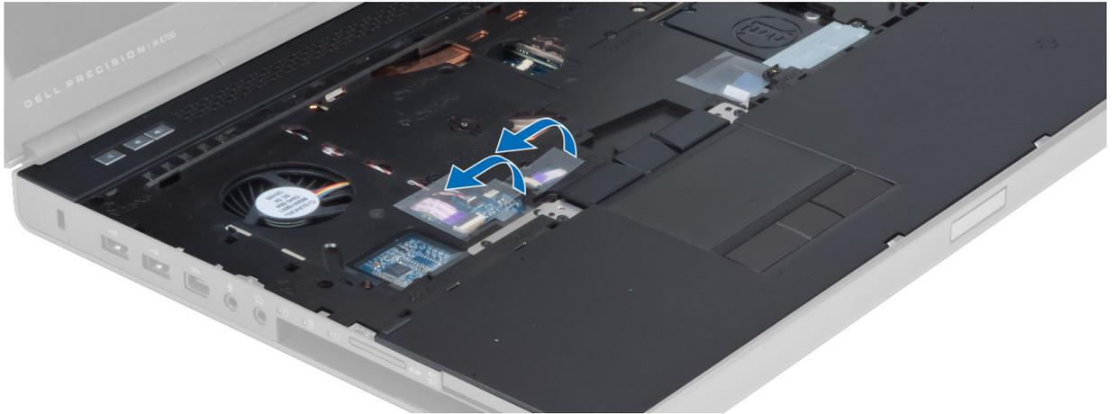
7. Disconnect the media board cable and the speaker cable from the system board.
