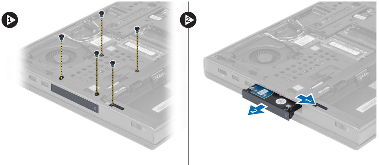
4. Flex the hard-drive bracket outward and pull out the hard drive from the bracket.
