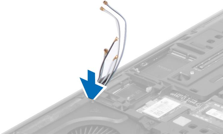
4. Flip the computer and pull up the antenna cables through the routing hole.
