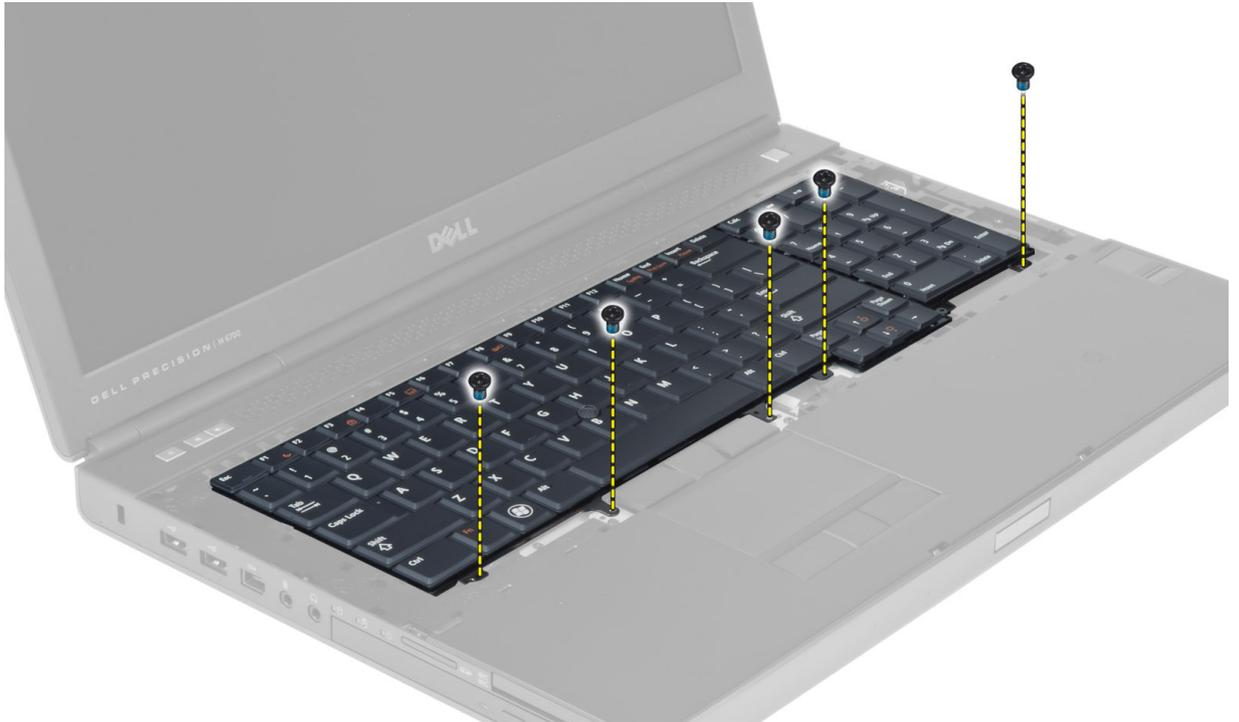
4. Starting from the bottom of the keyboard, separate the keyboard from the computer and flip the keyboard over.
