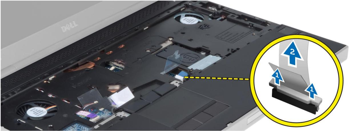
10. Disconnect the power button cable from the system board.
