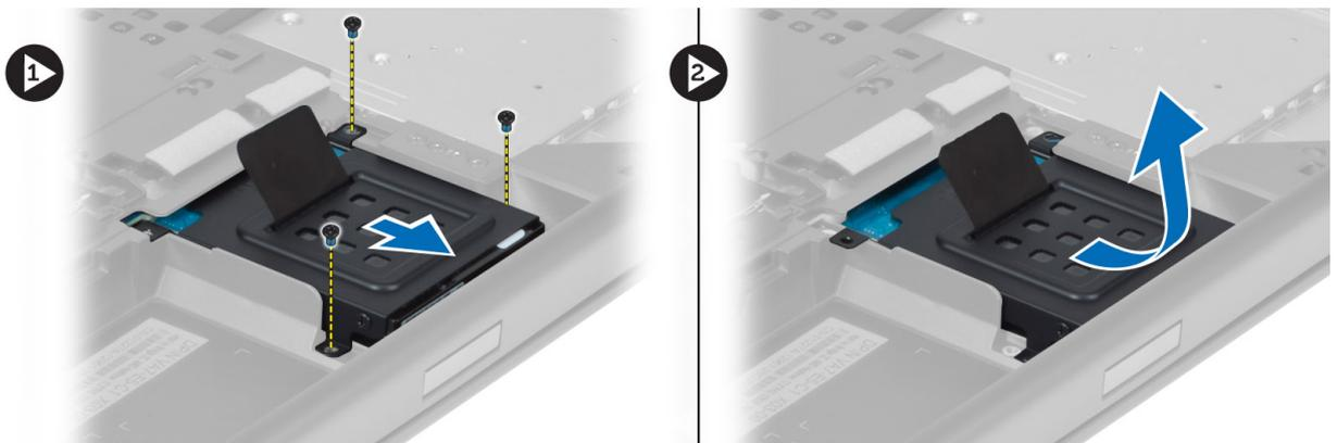
5. Remove the screw that secure secondary hard drive to the bracket.
