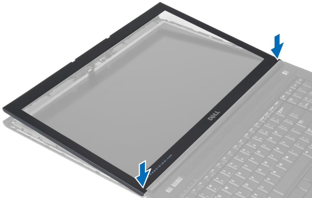
2. Work around the entire bezel until it snaps onto the display assembly.
