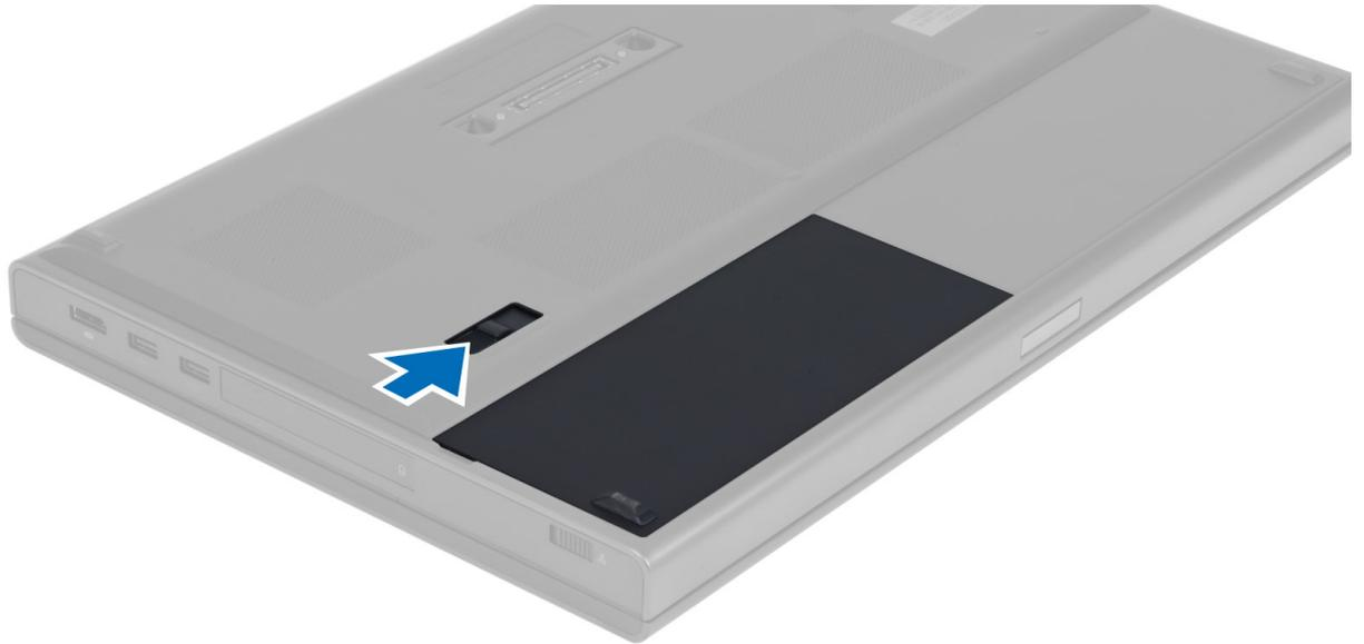
3. Flip and remove the battery from the computer.
