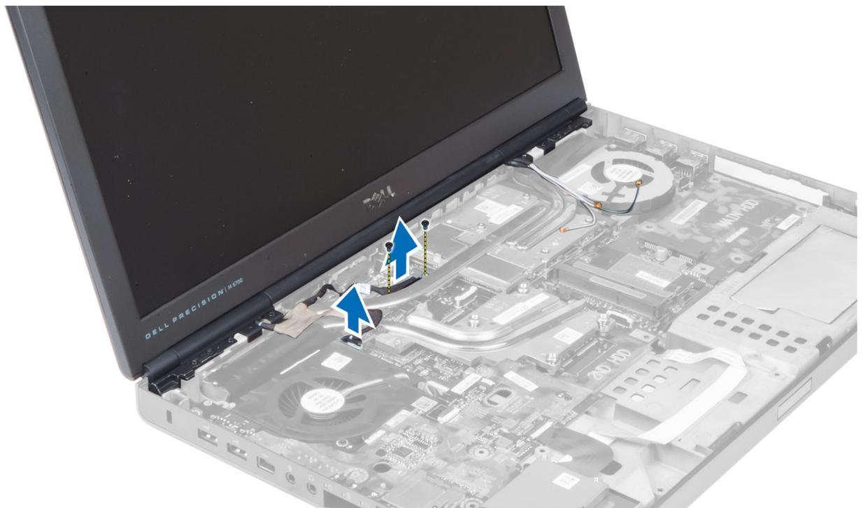
7. Remove the screws that secure the display assembly to the computer. Remove the display assembly from the computer.
