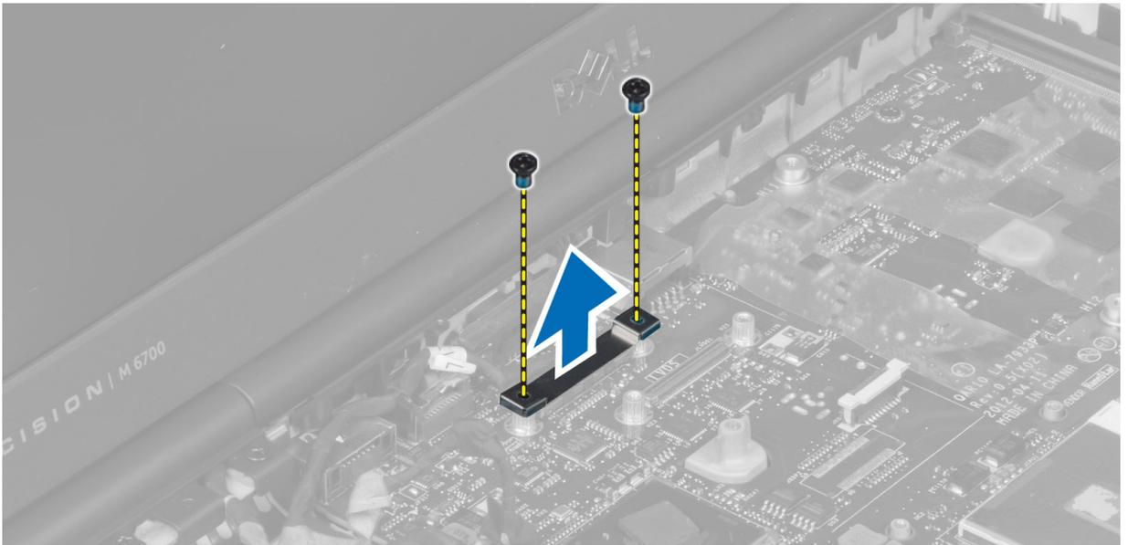
5. Disconnect the LVDS , camera and power connector cables from the system board.
