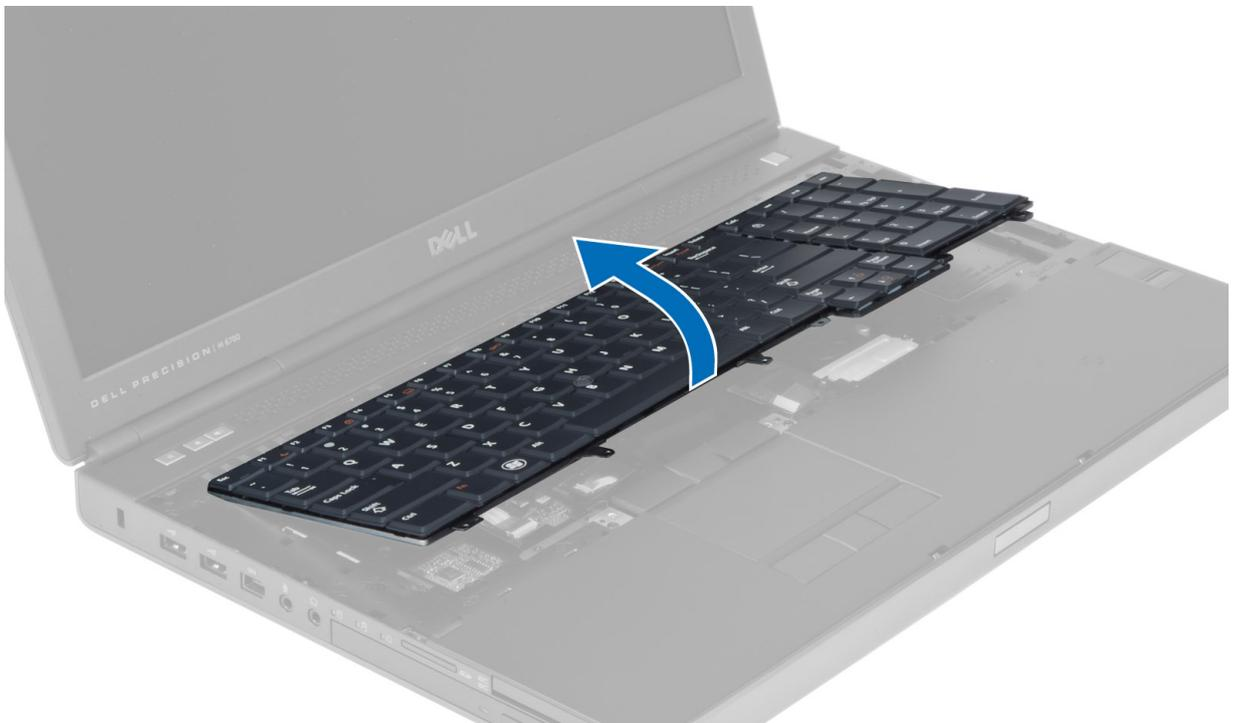
5. Disconnect the keyboard-data cable from the system board and remove the keyboard.
