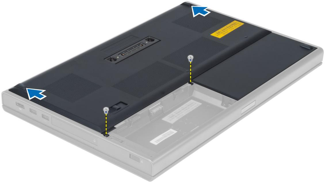
4. Flip and remove the base cover from the computer.
