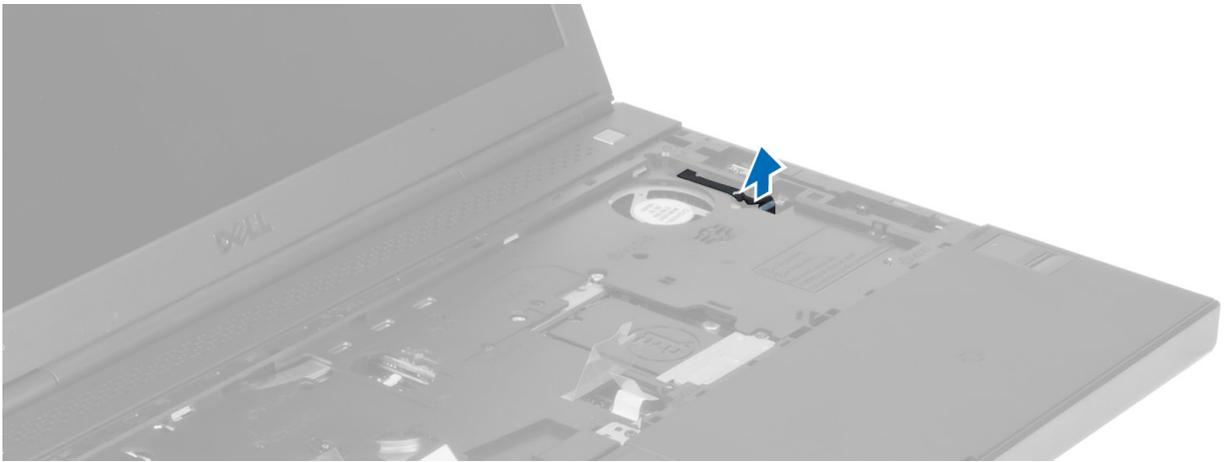
11. Disconnect the bluetooth module cable from the system board.
