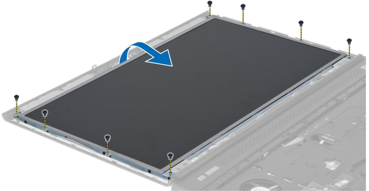
4. Peel back the adhesive tape that secures the LVDS cable to the display panel.
