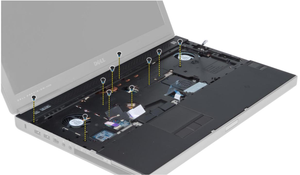
13. Lift the left edge of the palmrest. Release the tabs on the right edge of the palmrest and remove the palmrest from the computer.
