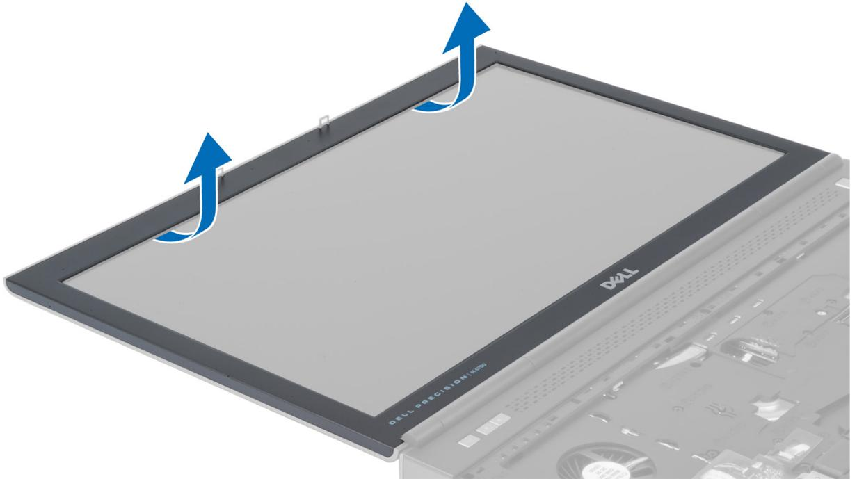
4. Work your way around the sides and top edge of the display bezel and remove the display bezel from the computer .
