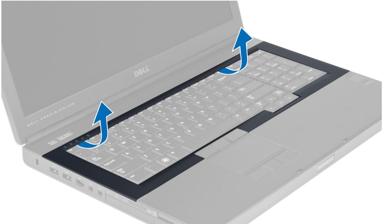
4. Pry up the bottom edge of the keyboard trim from the top-inner edge.
