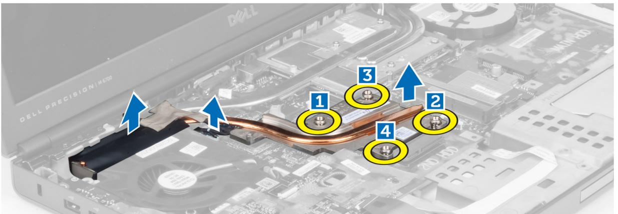
4. Remove the heat sink from the computer.
