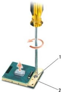
1 ZIF-socket cam screw 2 ZIF socket
