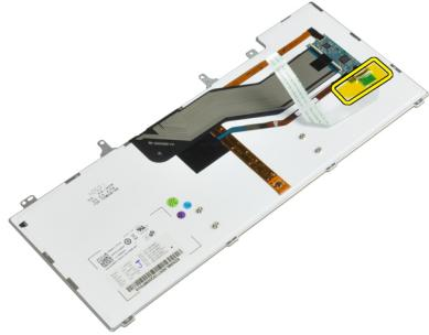
9. Uklonite kabel tipkovnice s tipkovnice.
