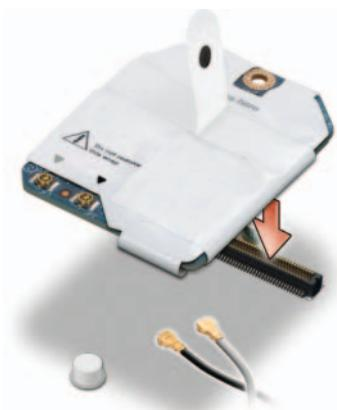
**NOTE:** If you are replacing an existing Latitude ON card, disconnect the attached cables and loosen the screw. Then, lift the card out of its connector by pulling the tab away from the computer.
