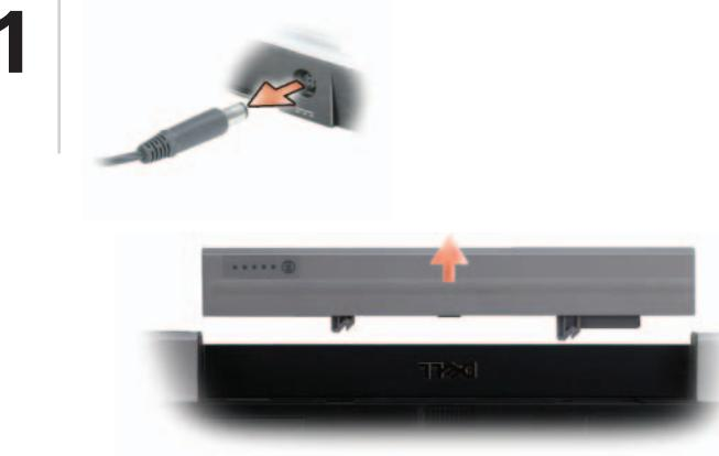
Disconnect the AC adapter and battery.
