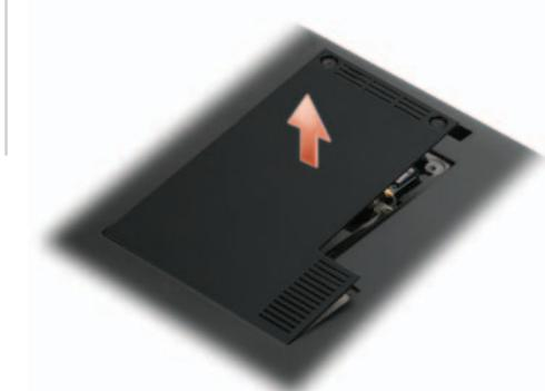
Remove the back cover to access the Latitude ON card slot.
