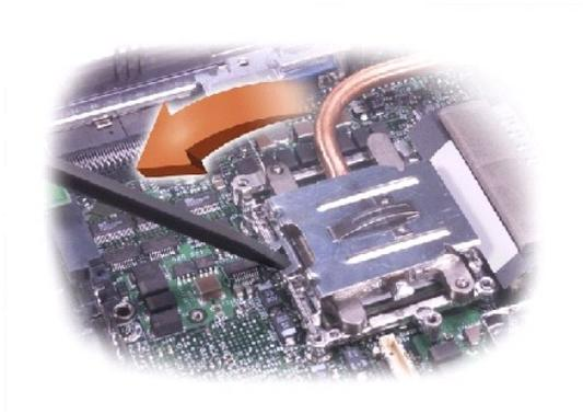
4. Close the microprocessor retaining clip.
