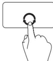
Move a finger in the horizontal scroll zone (extreme bottom of the touch pad), in a clockwise circular motion to scroll right or counterclockwise circular motion to scroll left.
