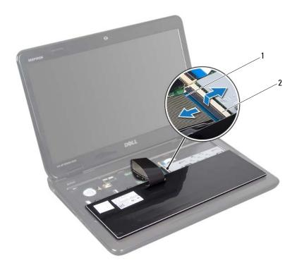
1 keyboard cable 2 keyboard-cable connector
