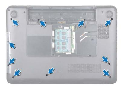
**7** Remove the five screws on the palm-rest assembly.
