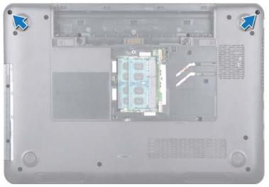
**9** Release the two tabs that secure the hinge cover to the computer base.
