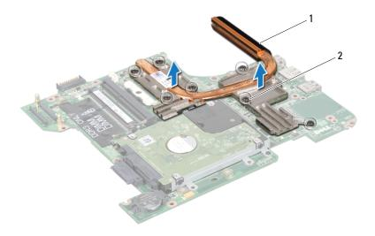
1 thermal cooling assembly captive screws (7)
