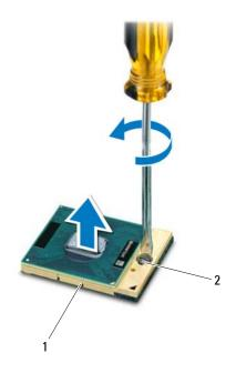
1 ZIF socket 2 ZIF-socket cam screw
