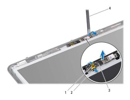
1 tape 2 camera cable 3 camera module 4 plastic scribe
