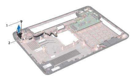
1 screw 2 AC-adapter connector cable
