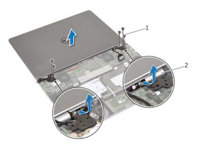
1 screws (5) 2 display-hinges (2) 7 Remove the display assembly from the palm-rest assembly.
