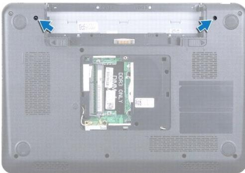
6. Remove the keyboard (see [Removing the Keyboard](#)).
