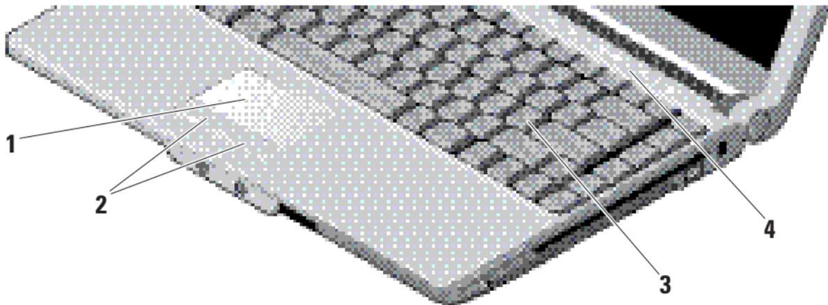
**1 Touch pad** – Provides the functionality of a mouse to move the cursor, drag or move selected items, and left-click by tapping the surface.
