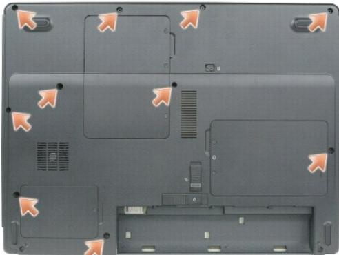
8. Turn the computer top-side up and remove the five M2.5 x 5-mm screws from the top of the palm rest and the remaining two M2.5 x 3-mm screws from near the power button and the activity LEDs.
