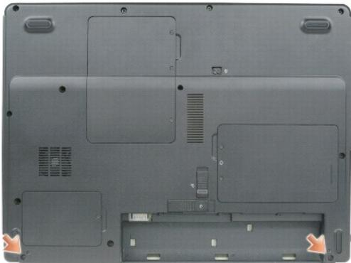
9. From the back of the computer, remove the two M2.5 x 8-mm screws labeled "D."
