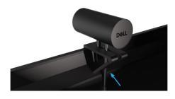
**5.** Remove the magnetic lens cap and place it at the rear of the webcam.
