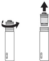
3. Install the coin-cell batteries into the coin-cell battery holder.
