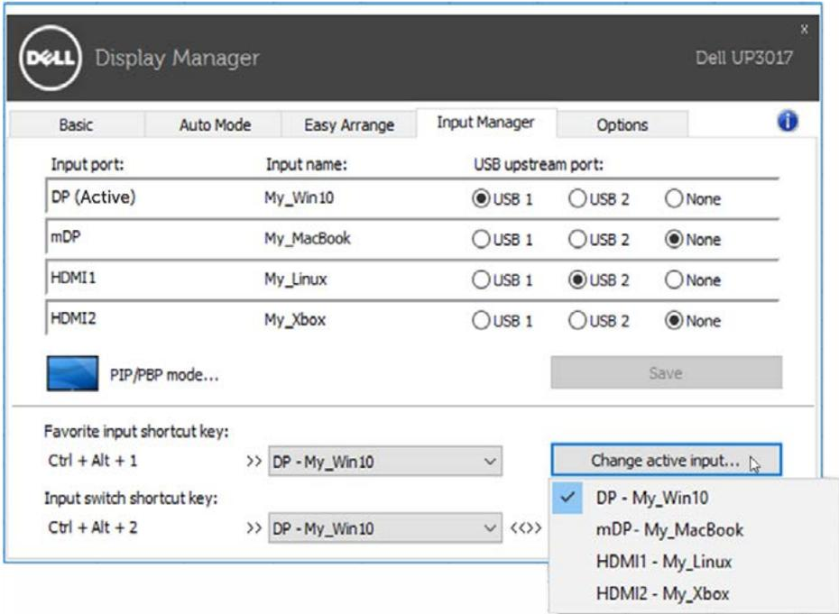
**NOTE:** DDM communicates with your monitor even when the monitor is displaying video from another computer. You can install DDM on the PC you frequently use and control input switching from it. You may also install DDM on other PCs connected to the monitor.
