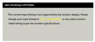
This means that the monitor cannot synchronize with the signal that it is receiving from the computer. See Monitor Specifications for the Horizontal and Vertical frequency ranges addressable by this monitor. Recommended mode is 2560 x 1440.
