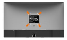
**NOTE:** Use M4 x 10 mm screws to connect the monitor to the wall-mounting kit. Refer to the instructions that come with the VESA-compatible wall mounting kit.
