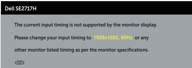
This means that the monitor cannot synchronize with the signal that it is receiving from the computer. See [Monitor specifications](#) for the Horizontal and Vertical frequency ranges addressable by this monitor. Recommended mode is 1920 x 1080.
