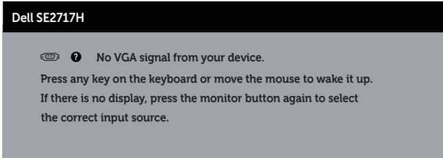
If VGA or HDMI cable is not connected, a floating dialog box as shown below appears. The monitor will enter Power Save Mode after 4 minutes if left at this state.
