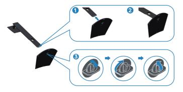
**5.** Slide the tabs on the stand assembly into the slots on the monitor and press the stand assembly down to snap it into place.
