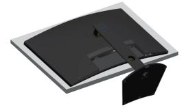
2. Press and hold the stand release button, and then lift the stand off the monitor.
