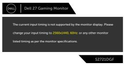
This means that the monitor cannot synchronize with the signal that it is receiving from the computer. See **Monitor Specifications** for the Horizontal and Vertical frequency ranges addressable by this monitor. Recommended mode is 2560 x 1440. You can see the following message before the DDC/CI function is disabled:
