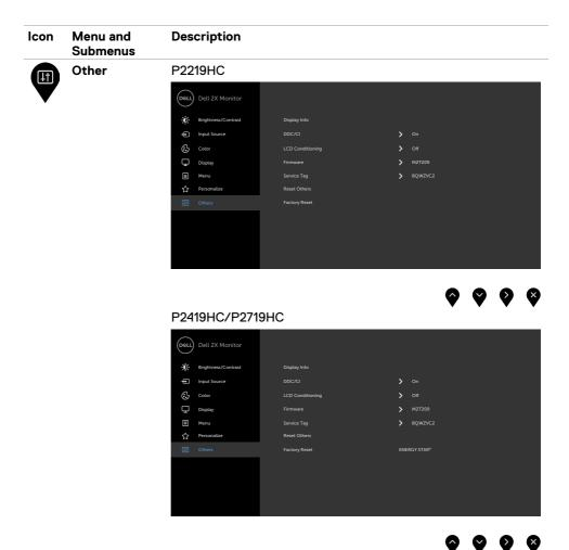
Select this option to adjust the OSD settings such as the **DDC/CI, LCD conditioning,** and so on.
