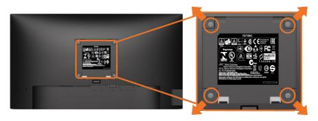
**W** NOTE: Use M4 x 10 mm screws to connect the monitor to the wall-mounting kit.
