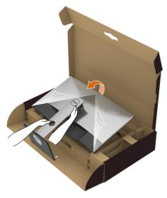
**NOTE:** Lift the monitor carefully to prevent it from slipping or falling.
