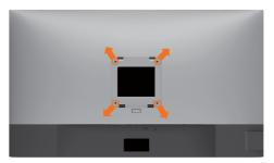
**NOTE:** Use M4 × 10 mm screws to connect the monitor to the wall-mounting kit.
