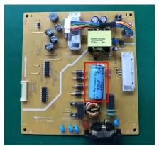
S1 -1 Cut the glue between bulk cap. and PCB with a knife
