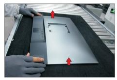
S7 Lift the rear cover up carefully. Disconnect the USB FFC cable from the connector of the interface board, and then remove the rear cover.
