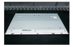
Turn over the bracket chassis module. Remove the Mylar from the hooks of the bracket, and then use a Philips-head screwdriver to remove two screws for unlocking AC power outlet.
