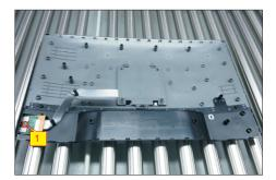
Tear off 2pcs aluminium foils for unfixing the bracket, then tear off 1pcs mylar tape, and then tear off 1pcs acetate tape for unlocking the panel lamp cable.
