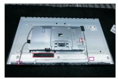
Use a Philips-head screwdriver to remove 5pcs screws for unlocking the front bezel with the assembled unit.
