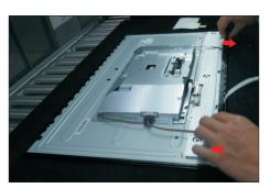
Tear off the mylar tape on the function key board, then use a Philips-head screwdriver to tighten 3pcs screws for locking the function key board with the front bezel.
