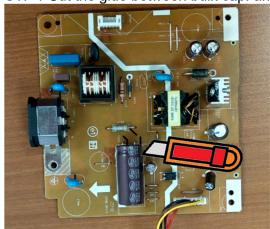
S17-2 Ensure cutting path within the glue, don't touch bulk cap. or PCB
