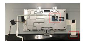
S8 Remove 1 tape from Backlight Wire
