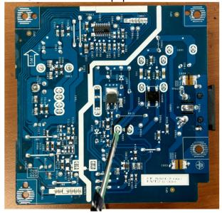
S18-4 Lift the bulk cap. up and away from the PCB
