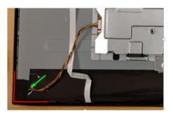
S9 Disassemble Backlight Wire from panel and SPS BD
