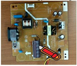
S17-3 Take out bulk cap. pin solder with soldering iron and absorber
