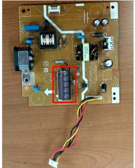
S17-1 Cut the glue between bulk cap. and PCB with a knife
