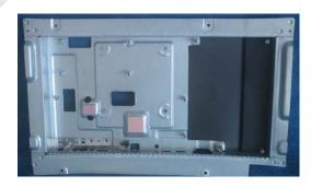
Use a Philips-head screwdriver to remove 15 screws for unlocking the middle plastic bezel with the whole unit, and then remove the middle plastic bezel carefully.
