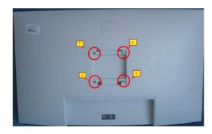
Wedge your fingers between the rear cover and the middle bezel on the corners of the top side of the monitor to release the rear cover, then use one hand to press the middle bezel, the other hand to pull up carefully the rear cover in order of arrow preference for unlocking mechanisms of rear cover
