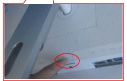
Remove the screw to remove the stand assy and the base assy.
