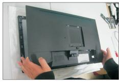
Remove the rear cover. Tear off the aluminum foil, and then disconnect the USB cable and Function key cable away from the connector of the interface board. Use a Philips-head screwdriver to remove one screw for unlocking the USB unit, remove the USB unit from the hooks.
