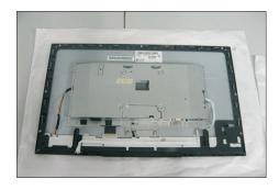
Use a Philips-head screwdriver to remove four screws for unlocking the bracket chassis module S8 with the panel module.
