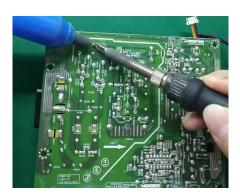
S15-5 Lift the bulk cap. up and away from the PCB
