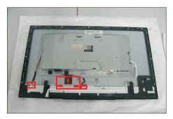
Use a Philips-head screwdriver to remove nine screws for unlocking the middle bezel with the assembled unit. Use a Philips-head screwdriver to remove two screws for unlocking the front bezel. Put the bracket chassis module on the protector.
