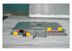
Turn over the bracket chassis module. Remove the Mylar from the hooks of the bracket, and then use a Philips-head screwdriver to remove six screws for unlocking the interface board and power board.
