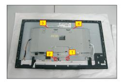
Disconnect the panel power cable to the connector of the panel module. Then disconnect the other cables S9 as the below picture shown.
