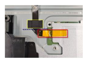
S12 Unlock 19 screws to disassemble Middle Frame from Panel
