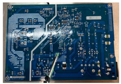
S18-4 Lift the bulk cap. up and away from the PCB
