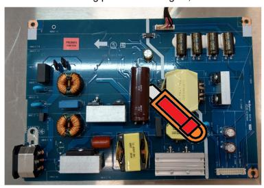
S18-3 Take out bulk cap. pin solder with soldering iron and absorber
