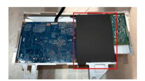
S15 Unlock 10 PCBA screws to disassemble "I/F BD", "SPS BD" and "LED Driver BD" from Main SHD
