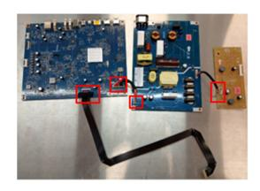
Remove electrolyte capacitors (red mark) from printed circuit boards
