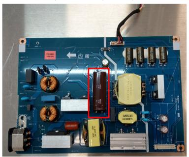
S18-1 Cut the glue between bulk cap. and PCB with a knife
