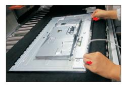
Tear off the mylar tape on the function key board, then use a Philips-head screwdriver to tighten 3pcs screws for locking the function key board with the front bezel.
