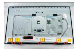
Use a Philips-head screwdriver to remove 2pcs screws(left and right) for unlocking the front bezel with the panel module, then disassemble the front bezel with the unit and put it aside.
