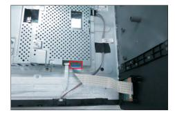
Use a Philips-head screwdriver to remove one screw for unlocking the USB board unit, then release the USB board unit and put it aside.
