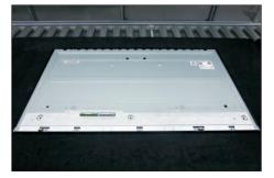
Turn over the bracket chassis module. Remove the Mylar from the hooks of the bracket, and then use a S17 Philips-head screwdriver to remove two screws for unlocking AC power outlet.
