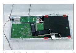
Use a Philips-head screwdriver to remove 7pcs screws for unlocking power board and interface board and driver board.
