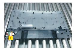
Tear off 2pcs aluminium foils for unfixing the bracket, then tear off 1pcs acetate tape for unlocking the panel lamp cable.
