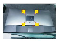
Wedge your fingers between the rear cover and the middle bezel on the corners of the top side of the monitor to release the rear cover, then use one hand to press the middle bezel, the other hand to pull up carefully the rear cover in order of arrow preference for unlocking mechanisms of rear cover.
