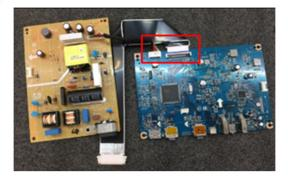
**S17** Remove electrolyte capacitors (red mark) from printed circuit boards
