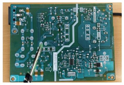
S17-3 Take out bulk cap. pin solder with soldering iron and absorber
