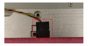
S13 Disassemble 5 plastic BOSS from panel
