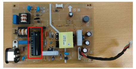
S17-1 Cut the glue between bulk cap. and PCB with a knife
