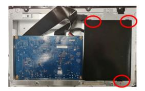
**S15** Unlock 8 PCBA screws to disassemble I/F BD, SPS BD from Main SHD
