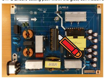
S17-3 Take out bulk cap. pin solder with soldering iron and absorber
