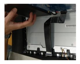
S11 Unlock 14 screws to disassemble Middle Frame
