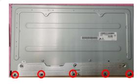
\$14 Disassemble mylar from Main SHD
