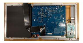
S15 Unlock 10 PCBA screws to disassemble I/F BD, SPS BD and LED Driver BD from Main SHD
