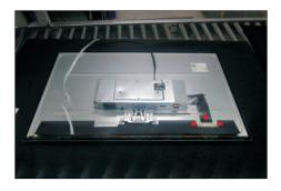
S10 Lift up the bracket chassis and put it on a protective cushion.
