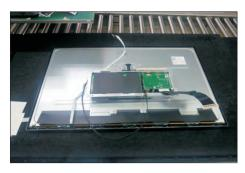
Release the panel module away from the hooks of the front bezel, then lift up the panel module and take away the front bezel with key board.
