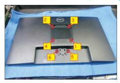
Turn over the LCD monitor to let the screen faced up, place a cloth on the panel where you are working on to protect the panel. Continually, wedge your fingers between the front bezel and the panel in order of arrow preference for unlocking mechanisms. Turn over the LCD monitor to let the screen faced down and then remove the rear cover.
