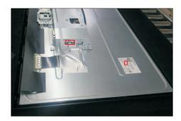
Tear off 2pcs aluminum foils for unlocking panel lamp cable and LVDS cable, and then disconnect the panel lamp cable away from the connector of panel module.
