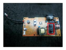
S16-1 Cut the glue between bulk cap. and PCB with a knife.
