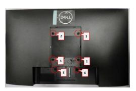
4. Tear the aluminum foil & remove the cable
