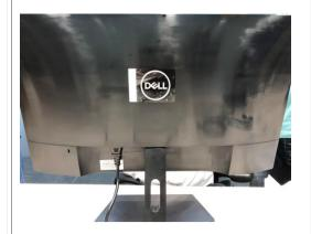
Press upper edge of the back cover (start with top of monitor) with both thumbs, the rest 4 fingers pull back cover upwards. Repeat the action 2-8 position to remove back cover.
