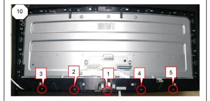
Use a Philips-head screwdriver to remove 5 screws to remove the DECO\_BEZEL. (No.1~5 screw size=M2x2.5, Torque=1±0.2kgf.cm)
