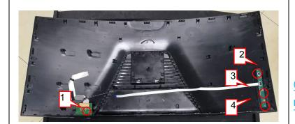
Use a Philips-head screwdriver to 1 screw to unscrew USB board and remove 3 screws for unlocking the key board (No.1~3 screw size=Q3x6, Torque=4±1kgf.cm No.2~4 screw size=M2.5x2, Torque=0.9±0.4kgf.cm)
