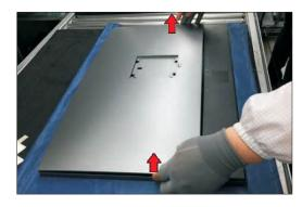
Remove the rear cover and put it on a protective cushion. Use a Philips-head screwdriver to remove 20 screws for unlocking the middle plastic bezel with the whole unit, and then remove the middle plastic bezel carefully.
