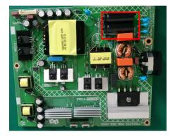
Take out bulk cap. Pins older with soldering iron and absorber.
