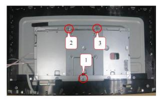
Remove the Mylar. Use a Philips-head screwdriver to remove 4 screws for unlocking the main board and the adapter board
