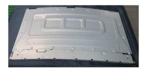
Use a Philips-head screwdriver to remove 4 screws for unlocking the key board and the middle frame. Disconnect the pin.
