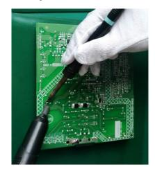
Lift the bulk cap. up and away from the PCB
