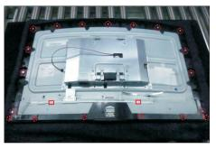
Remove the middle bezel and put it into a fixture jip, then tear off the tape for releasing the touch key board away from the middle bezel. Tear off the black PVC tape and use a Philips-head screwdriver to remove 1pcs screw for unlocking the power key board with the front bezel.
