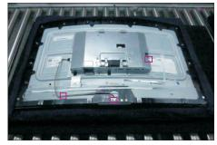
Tear off 2pcs tapes of the power cable. Use a Philipshead screwdriver to remove 6pcs screws for unlocking the middle bezel with the front bezel. Use a Philipshead screwdriver to remove 13pcs screws for unlocking the middle bezel with the panel module.
