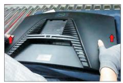
function key cable and LED cable from the connectors of the interface board, and then remove the rear cover.
