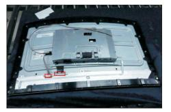
Use a Philips-head screwdriver to remove 6pcs screws for unlocking the middle bezel with the front bezel. Use a Philips-head screwdriver to remove 13pcs screws for unlocking the middle bezel with the panel module. tear off 2pcs tapes of the power cable. (No.1~6 Screw size=M2x3.8,Torque=3±0.5kgfxcm; No.7~19 Screw size=M3x5, Torque=3~4kgfxcm)
