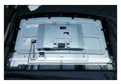
Put the rear cover on a protective cushion. Use a Philips-head screwdriver to remove 4pcs screws for unlocking the function key board with the rear cover. Tear off the key tapes and release the function key board from the hook of the rear cover.
