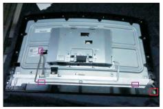
Use a Philips-head screwdriver to remove 4pcs screws for locking the bracket chassis module with the panel.
