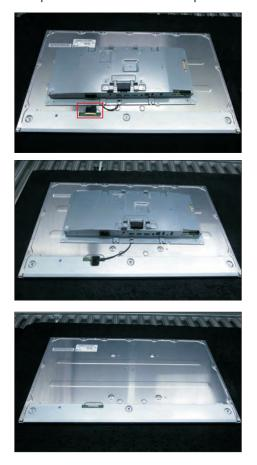
Turn over the bracket chassis module. Use a Philipshead screwdriver to remove 6pcs screws for unlocking power board and interface board, and then release the EDP cable from the hook of the bracket.
