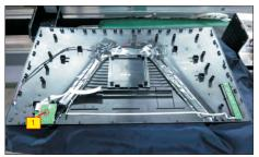
Use a Philips-head screwdriver to remove 4pcs screws for unlocking the joystick key board with the rear cover. Tear off the joystick key tapes and release the joystick key board from the hook of the rear cover. (No.1~4 screw size=M2x0.2, Torque= $0.8\pm0.2$ kgfxcm)
