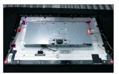
Tear off the mylar tape on the position as the picture below shown. Use a Philips-head screwdriver to remove 13pcs screws for unlocking the middle bezel with the panel module. Use a Philips-head screwdriver to remove 2pcs screws for unlocking the middle bezel with the front bezel.
