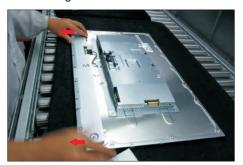
Use a Philips-head screwdriver to remove 4pcs
