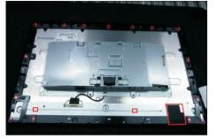
Remove the middle bezel and put it into a fixture jip, then use a Philips-head screwdriver to remove 1pcs screw for unlocking the power key board with the front bezel.
