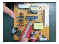
S19-3 Cut into the bottom of bulk cap. and pullit up carefully.
