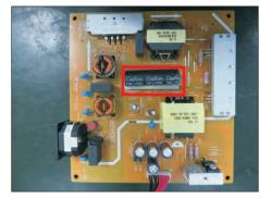
S19-1 Cut the glue between bulk cap. and PCB with a knife.
