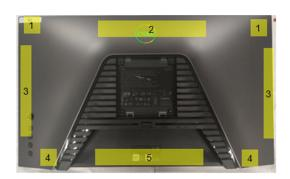
Remove CTRL BD FFC from I/F BD and remove all tapes from Main SHD
