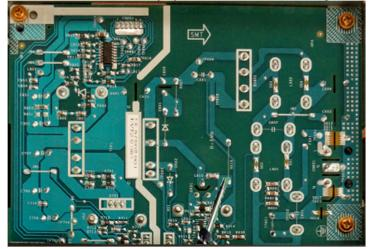
S30-4 Lift the bulk cap. up and away from the PCB
