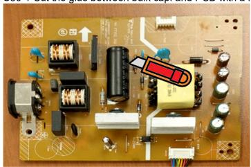
S30-2 Ensure cutting path within the glue, don't touch bulk cap. or PCB
