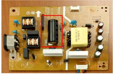
S30-1 Cut the glue between bulk cap. and PCB with a knife
