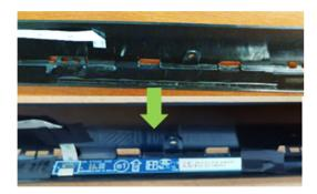
S23 Unlock 2 screws to disassemble BTN-PWR from Middle Frame
