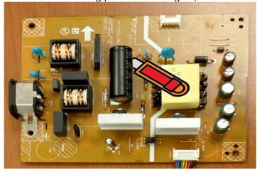
S30-3 Take out bulk cap. pin solder with soldering iron and absorber
