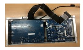
Remove "LVDS FFC cable" and "WIRE 6P/10P" from I/F BD
