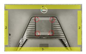
Remove "CTRL BD FFC" from I/F BD and tear off it from Main SHD to take off Rear Cover
