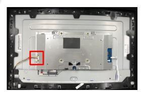
S11 Remove conductive cloth and acetate tape from panel
