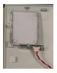
Remove FFC cables from Rear Cover, CTRL BD and CTRL+KEY BD
