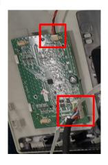
S13 Unlock 1 screw to disassemble LED Driver BD from Rear Cover
