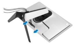
Disconnect the cables from the monitor and slide them out through the cable-management slot on the stand riser.
