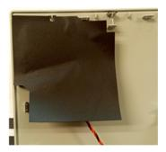
S15 Unplug wire from LED BD and disassemble LED BD from Rear Cover
