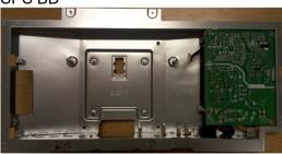
S36 Unlock the ground screw and disassemble power socket from SHD
